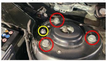
Lift plastic shroud to expose strut tower. Remove 3x strut mount bolts using M13 socket (red circles) and 1x firewall shroud nut (yellow circle) with M10 socket.
