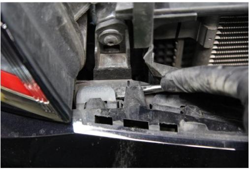
**Step 6:** Remove the foam crashbar. Measure 22.5" from the right side of the car and mark the center line.
