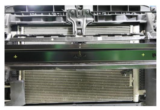
**Step 9:** Center-punch and drill mounting holes. Start with a small drill bit and work your way up to 19/64". Be careful not to damage the A/C condenser.
