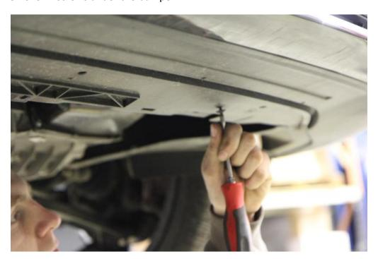
**Step 5:** Remove the bumper. Pull off the sides of bumper from the wheel well. Unclip the retaining tabs next to each headlight. Pull bumper forward and free from the car. Disconnect foglight harnesses.
