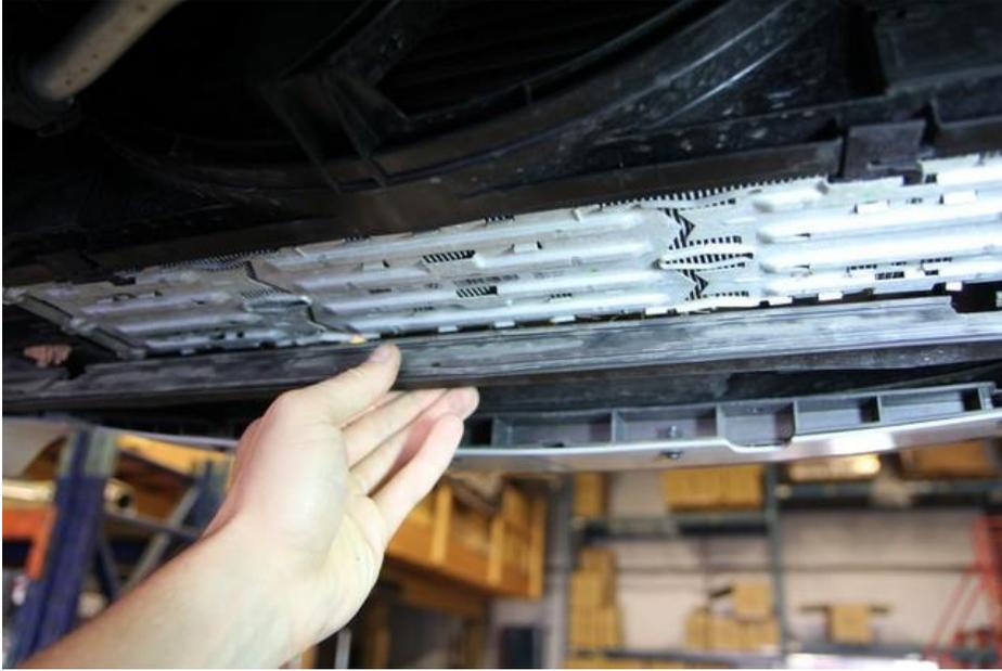
Step 3: Push the plastic cover down and lower the factory intercooler (will not be reused). Pull down carefully. Remove charge pipes and take out the factory intercooler.
