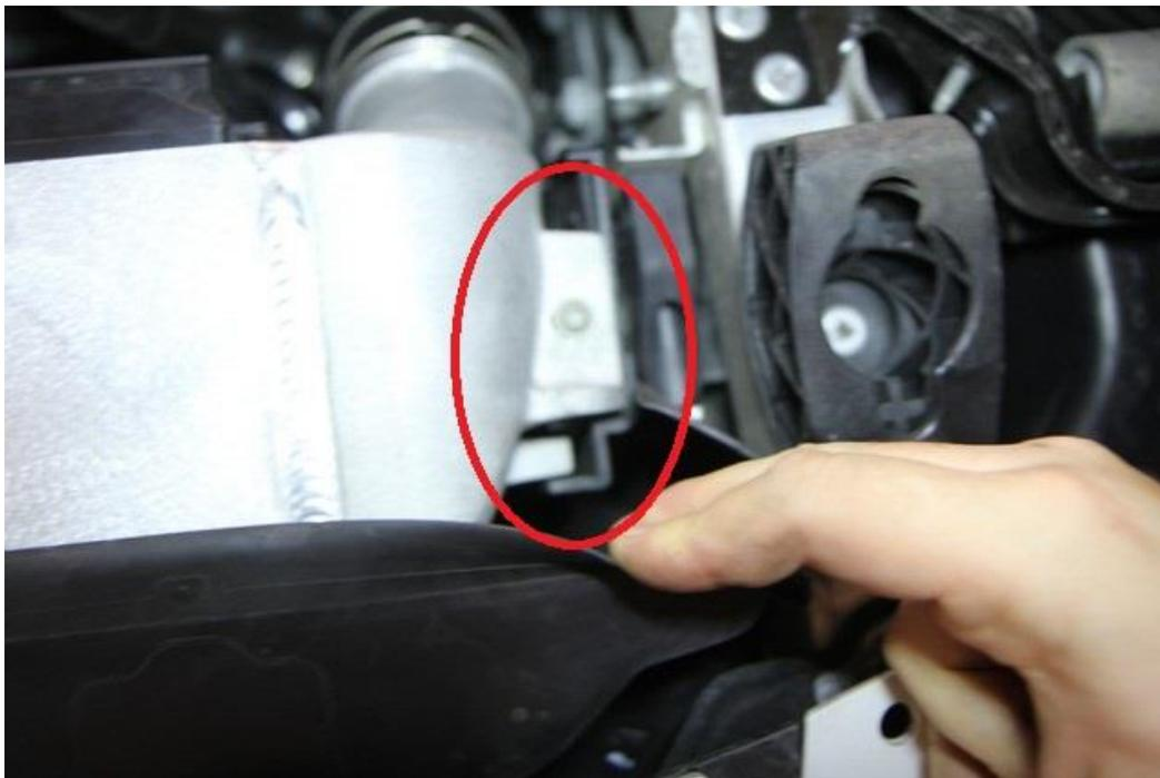
Step 5: Clip in charge pipes and reinstall bellypan. Test drive vehicle.
