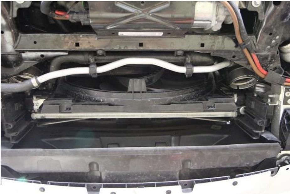
Step 4: Following the same procedure, reinstall CTS Turbo intercooler. Make sure the intercooler tabs line up with plastic guides. Secure intercooler using factory T25 torx screws.
