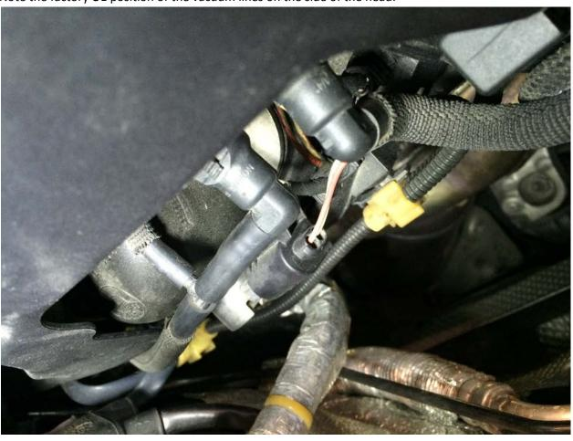
Install provided T in vacuum lines on passenger side of engine as pictured. This requires no cutting, but the factory vacuum lines pictured above are tight on the vacuum fittings and may require some persuasion with a small pick. The long vacuum line below will connect to the included solenoid on the "grey" end, which runs parallel to the nipple barb on the black end of the solenoid.
