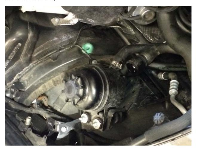
Remove 3 x 10mm nuts from back of wastegate actuator using ratchet & socket.
