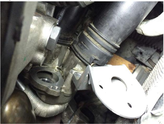
Install CTS BOV in place of the OE valve with nipples oriented as below, using CTS provided mounting allen head bolts using ratchet, bit and extension. Install included vacuum lines on BOV barbed nipples. Please ensure the included O-ring is seated snugly on the base of the BOV at the connection between turbo/CTS BOV.
