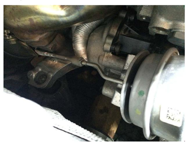
Remove 2 x Torx bolts holding wastegate actutor bracket to turbo to gain additional clearance to valve. Or remove one torx bolt, loosen the other and rotate the wastegate actutor bracket away from the OE valve.
