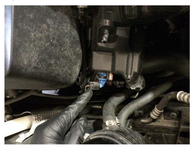
Pinch off coolant reservoir feed line, and coolant reservoir return line, remove coolant reservoir feed/return lines by depressing clips and drain coolant from reservoir, and tuck the just removed coolant hoses out of the way.
