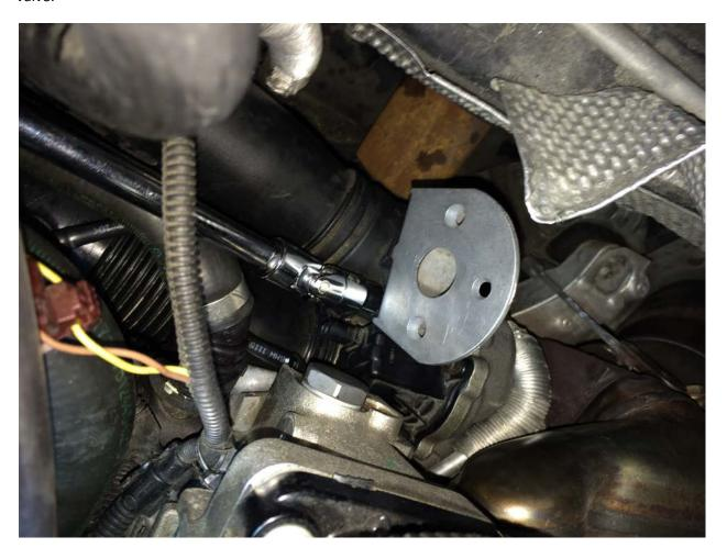
Remove 3 bolts holding in the factory recirculation (diverter valve) using ratchet & extension.
