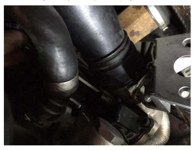
With the factory valve removed it should look as follows, notice we only removed one torx bolt from the wastegate bracket, and twisted the bracket to the side to gain additional clearance for valve removal.
