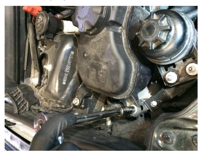
Unclip sensor from bottom of coolant reservoir
