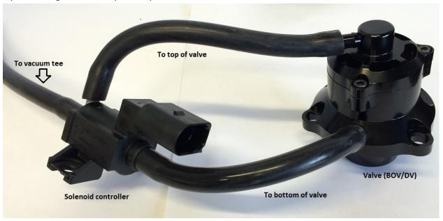
Install the electrical connector to the solenoid, it should clip in with a positive "clip" sound. Use spades and wire taps to connect to the OEM BOV electrical connection as pictured below, and cover the lines with sheathing. The OEM signal is now directed to the provided external solenoid in the top right of the picture, which now relays commands to the BOV that are sent from the factory DME/ECU. You can secure the solenoid valve under the edge of the OE engine cover for a stealth look.
