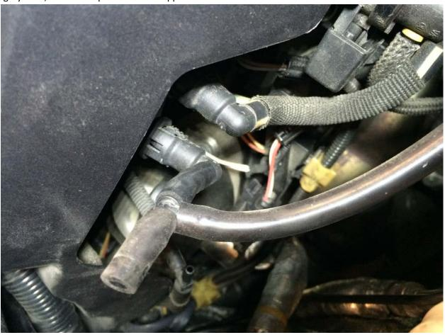
The vacuum lines should be routed as follows, pay particular attention to the vacuum line position related to the solenoid or you'll be doing the connections again. The "To vacuum tee" line goes to the top of the engine from the prior step.
