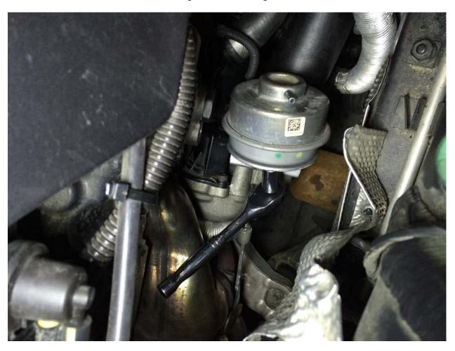
Mark jam nut on wastegate actuator, loosen the jam nut on the wastegate actuator rod, this should only require 1/4-1/2 of a turn. Once the wastegate rod jam nut is loosened pull back on the large head of the wastegate actuator and twist it counter clockwise, rotate the wastegate actuator until it comes free of the wastegate rod. Then remove the actuator.
