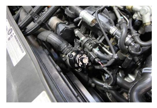
**Step 6:** Insert the included boost tap as shown and reattach the pcv clip on line. (not shown on this vehicle due to aftermarket catch can)
