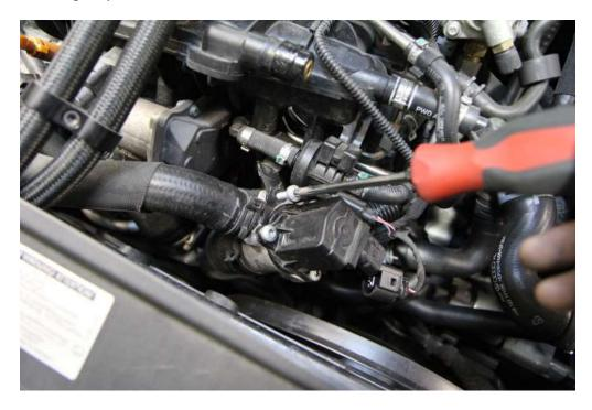
**Step 4:** Undo the 3 T25 Torx bolts holding the diverter valve to the vehicle.
