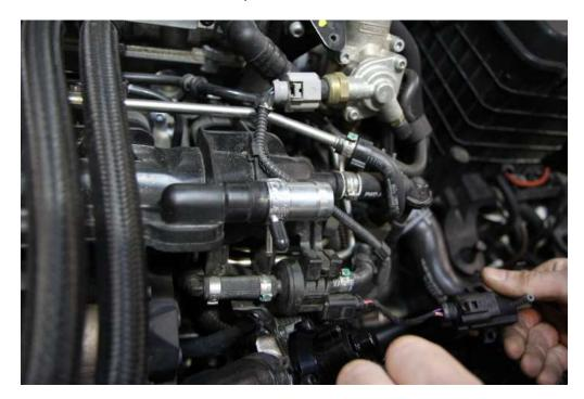
**Step 7:** Install the diverter valve plug into the included solenoid.
