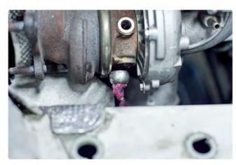
11) Remove rubber turbo coolant line from front of engine.
