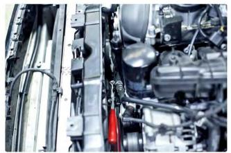
12) Once rubber turbo coolant line from front of engine is removed the line should look as follows.
