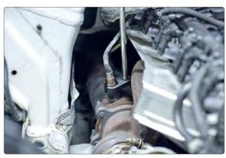
4) Remove downpipe from catalytic converter. Remove connectors from diverter valve, N75 valve, and oil sensor from oil pan.
