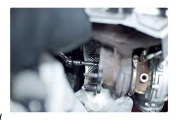
13b) Remove lower support bracket bolt and proceed to remove bracket.
