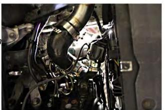
29) Re-install rear PCV between compressor housing and valve cover after completing modifications pictured below:
