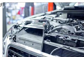
2) Remove airbox assembly and turbo inlet hose.
