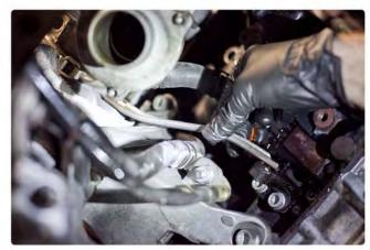
14) Remove the 5 upper exhaust manifold nuts. You do not need to remove the lower turbo bars or nuts along the lower portion of the exhaust manifold flange.
