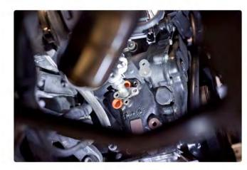
10) Remove coolant fitting from turbo.
