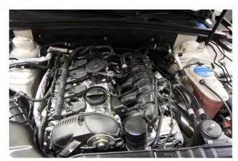
31) Re-install factory engine cover, replace engine oil and engine coolant. Ensure oil and coolant are topped up prior to starting vehicle. Bleed cooling system as per manufacturers specifications.
