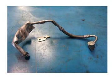
20a) Install modified coolant line onto new turbo with new crush washers supplied in kit.
