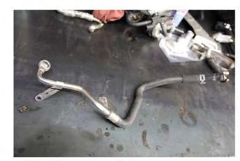
18b) This is the coolant line post modification. The bracket requires trimming as pictured.
