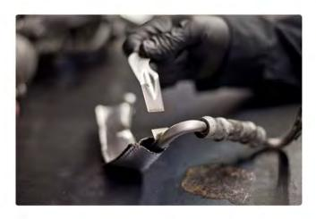
18a) Modify coolant line. This is the coolant line prior to modification.
