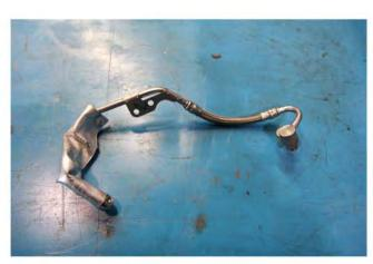
19b) This is the oil feed line, post modification. The bracket requires trimming as pictured.
