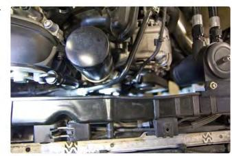
24) Install oil drain line on turbo and block. Install oil feed line onto the engine block.
