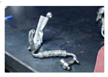
17b) This is the coolant line post-modification with bracket removed.
