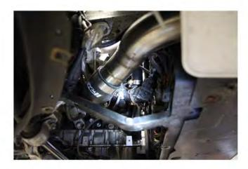
28) Install supplied 1" 90 degree elbow from compressor housing inlet and connect to side port on DV, then tighten clamps.
