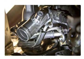
25) Install test pipe or optional high flow cat using the gaskets and hardware supplied in the kit.
