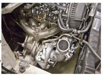
23) Reattach rubber end of coolant line to engine, this connection is pictured near the dipstick in the picture.
