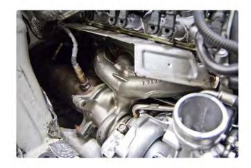
27) Install DV onto billet DV relocation falnge. Attach 1" 90 degree silicon to 1" bung on compressor outlet and onto bottom of DV relocation flange and tighten clamps.
