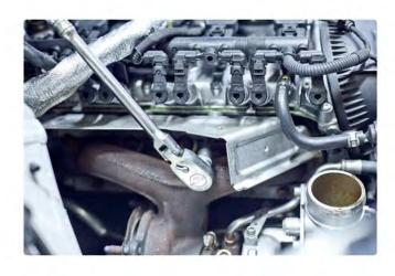
Pro Tip: turbo may need to be tapped upward to unseat from lower attachment bars.
