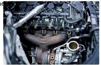
16) Remove turbo from car and place on work bench. Remove remaining water line and rear PCV connection from turbo.
