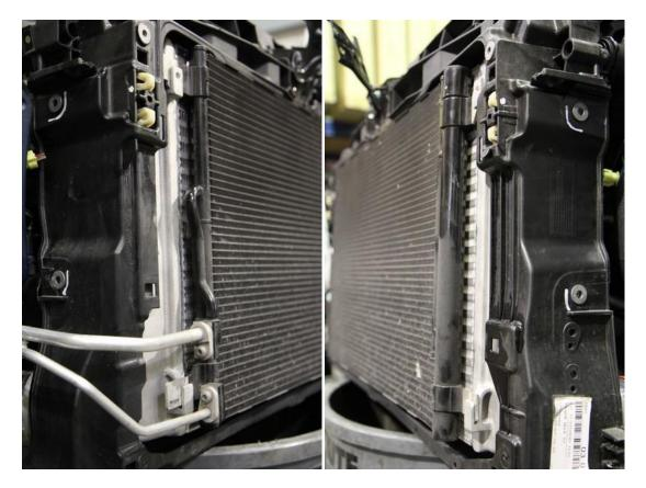
Step 10: Trim the plastic air deflectors where needed and re-install. Re-install crash bar and secure the radiator support. Install CTS FMIC hoses. Continue re-assembly by reversing the steps.
