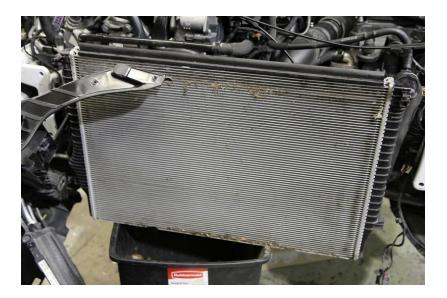
Step 10: Reinstall CTS Fmic into the factory location and make the necessary trimming on the radiator support (plastic) to accommodate for the larger intercooler. This is easily done using a Dremel tool and sidecutters if needed. Clearance on the A/C lines thru the rad support is needed as well and trimming the back part of the rad support.
