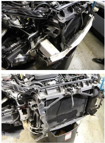
Step 8: Remove the factory clips holding the FMIC in place. WD40 is your friend here.
