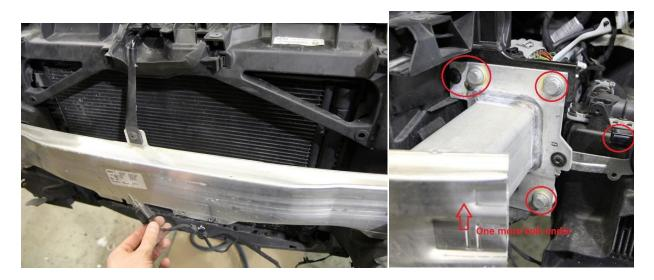
Step 7: Remove the rebar but tilting down and pulling the bar out.
