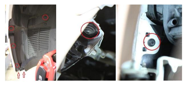
Step 2: Remove headlight washer line (squeeze the blue tabs), drain washer fluid and unclip the hose
