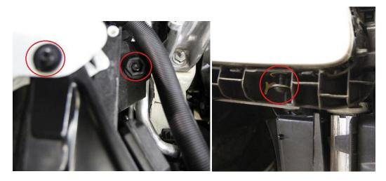
Step 5: Remove intake and front air scoop, T25 torx.
