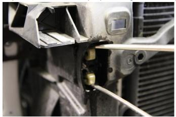
Step 9: Lift the intercooler and radiator assembly from the mounting holes on the bottom of the support and take off the support and A/C condenser. Move off to the left and unclip the factory intercooler at the top. Transfer mounting clips to CTS FMIC.
