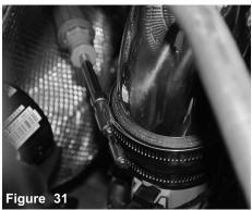
Now tighten the clamp on the turbo side using 8mm nut driver.
