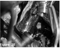
Install the intake tube into vehicle and position the tube to the step hose.
