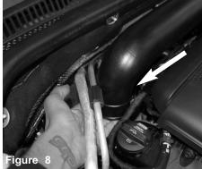
With pliers, carefully pull the intake tube out
