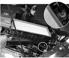
Loosen the bolt on the lower part of the airbox using T30 torx-bit. Carefully remove the lower part of the airbox out of vehicle including the drain line attached to the air box.
