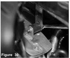
Tighten the remaining vibramount using 10mm socket or wrench.
