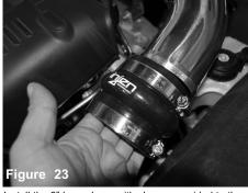
Install the 3" hump hose with clamps provided to the intake tube. Do not tighten.
