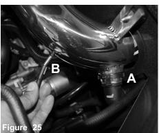
A) If equipped with smog pump, connect to the fitting on intake tube. if not equipped, use provided vinyl cap. B) Connect the factory vacuum line to the fitting on the intake tube.
