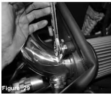
Now tighten the vibramount on the heat shield using 10mm socket or wrench.
