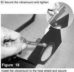
using provided M6 nut. Install the rubber trim seal to the top of the heat shield.
