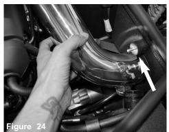
Install the second intake tube assembly into vehicle. connect the 2 tubes using hump hose. Do not tighten.
