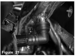
Connect the crankcase line to the fitting on intake tube. NOTE: Some light lubication on the inside will make for easy installation.
