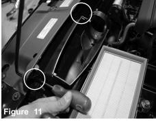
Loosen the 2 screws holding in the ram scoop using T25 torx bit or screwdriver. Save the screws for later install.
