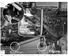
Now install the heat shield and position the tabs on heatshield to the factory ramscoop from step 11. Secure using factory screws. Tighten the rear tab using provided M6 allen screw and fender washer.
