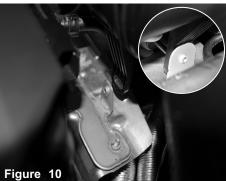
With T30 torx bit, loosen and remove the screw holding in intake tube neer fire-wall on engine.
