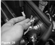
Secure the tab using provided m6 nut and fender washer. Do not tighten.
