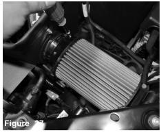
Install the air filter into vehicle and tighten using 8mm nut driver.
