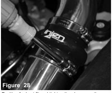
Position for best fit and tighten the clamps on the hump hose using 8mm nut driver.
