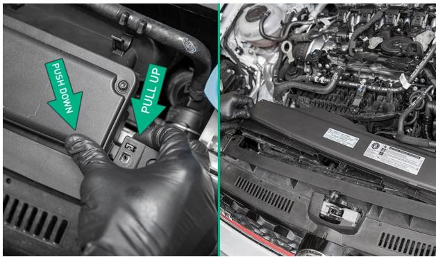
Once fully released from the radiator support, completely remove the airbox inlet from the vehicle.
