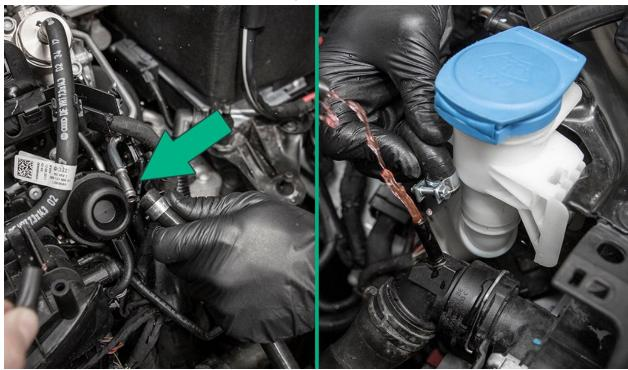
Once installed, firmly tighten both coolant line hose clamps.
