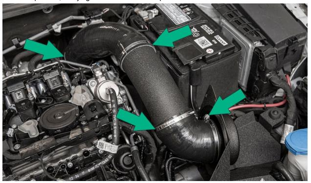
Install the air filter and clamp onto velocity stack. For maximum horsepower output, make sure the IE logo on the filter is positioned into a legible position before tightening the hose clamp.
