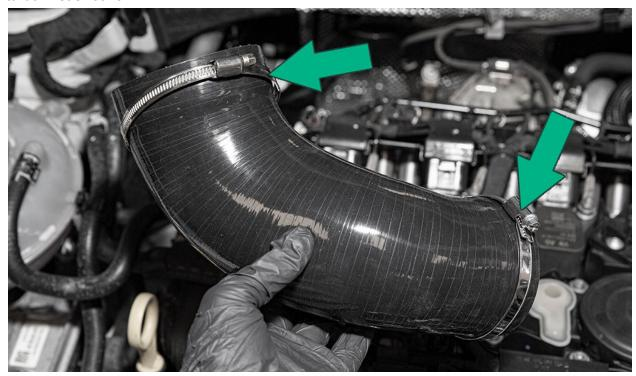
Assemble the long side of the IE turbo inlet pipe into the turbo side silicone hose. Orientate the silicone with the turbo and heat shield. *Do not tighten the hose clamps in this step.*
