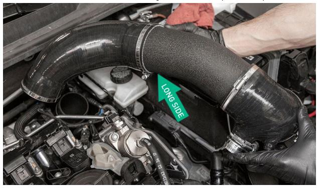
If equipped with SAI, push the SAI fitting onto the IE adapter until it clicks. Install the factory vacuum line onto the IE vacuum fitting barb.
