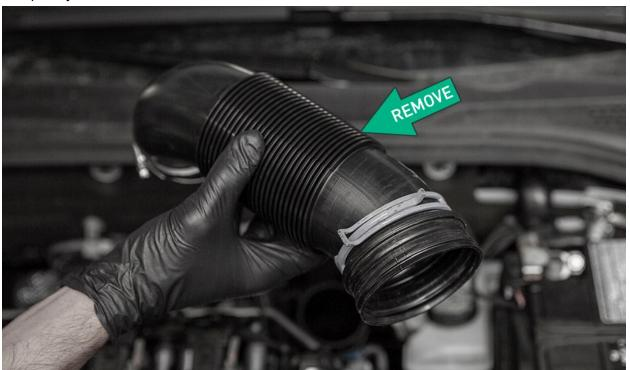
If your vehicle is equipped with secondary air injection (SAI), pinch the sides of the lock ring and pull back to disconnect it from the air box.
