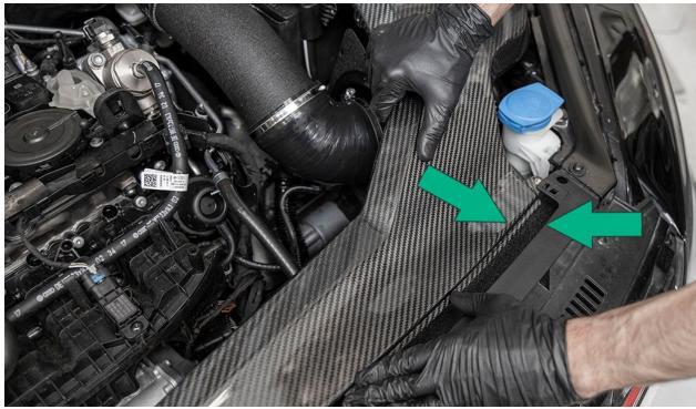
Install the 6 button head bolts and washers into through the slots on the IE heat shield and into the CF threaded inserts. We recommend starting on opposite ends of the cover and working in. Loosely install all bolts, and tighten once fully lined up and assembled. **Do not rush this step.**
