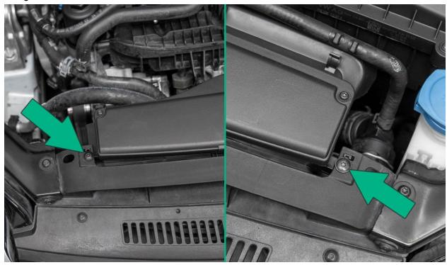
Push down on the inlet and carefully pull up on the lock tab to disconnect the front air box inlet. Repeat on both sides.
