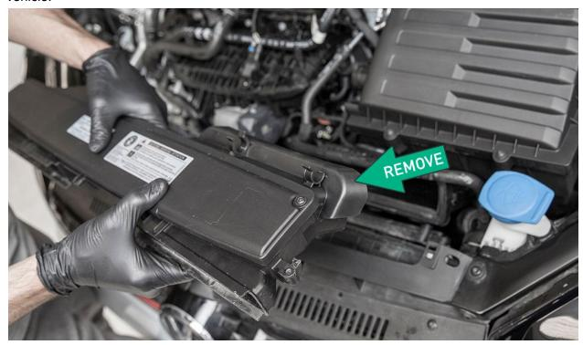
Pull up on the rubber mount grommet brackets (X2) to release and completely remove the airbox assembly from the vehicle. *Take special care not to break the plastic mount brackets.*
