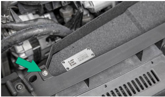
Firmly grasp the SAI filter line and with the opposite hand carefully rotate the SAI fitting 90 degrees clockwise rela the line. *If you do not have SAI, skip this step.*
