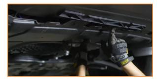
5. Remove the bolts that secure the lower and side edges of the bumper. (15x T25 torx bolts)
