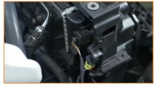
23. Separate the bumper support bracket that sits above the crash beam. (3x T30 torx bolts)
