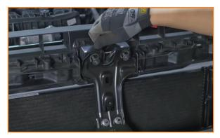
25. Move the ambient air temp sensor and emblem light sensor wiring harnesses that were unplugged earlier so they are out of the way.
