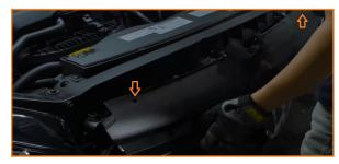
3. Disconnect the electrical harness at the back of the grille and remove the grille.
