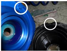
o Insert shock stud through the washer in the centre of TRC5000. Using the original fastener, tighten top mount down onto strut. Ensure notches are aligned.
