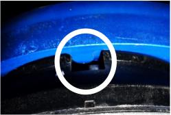
Install Strut into front of vehicle and use supplied fasteners to secure top of strut to the body. When both sides are installed, carry out a wheel alignment.
