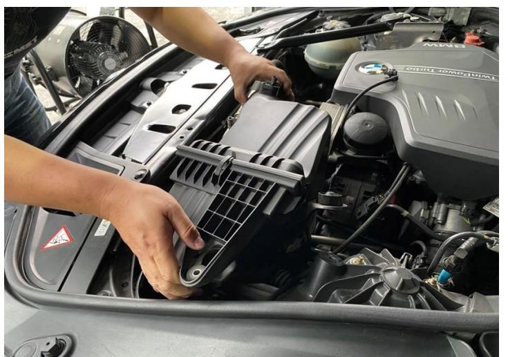
Figure 6: Remove the stock air box.
