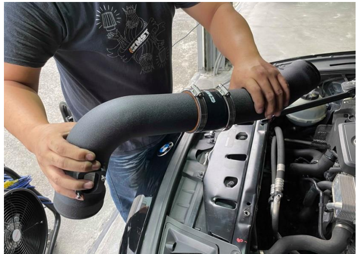
Figure 11: Install the intake pipe.
