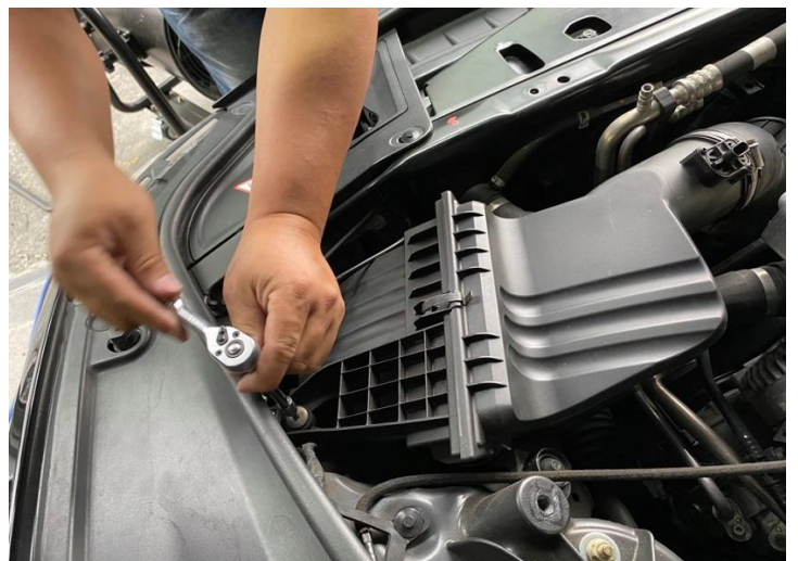
Figure 5: Remove the air box bolt.
