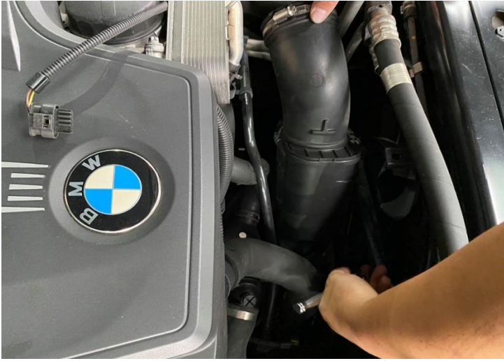
Figure 7: Remove the stock tube.
