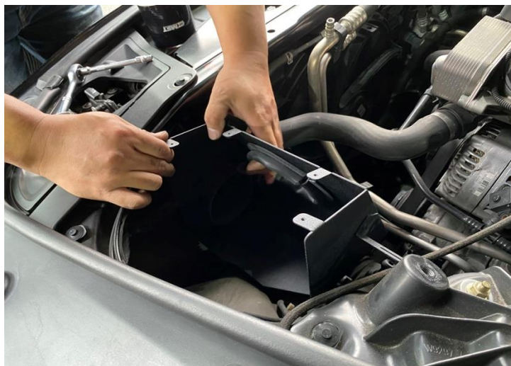
Figure 9: Install the heat shield.
