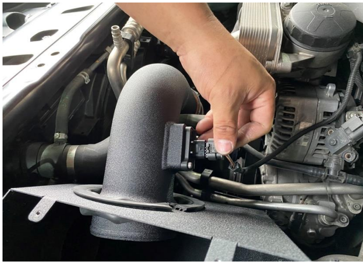
Figure 14: Connect the MAF sensor.
