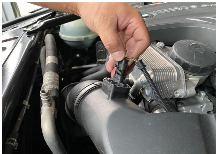
Figure 3: Disconnect the MAF sensor.
