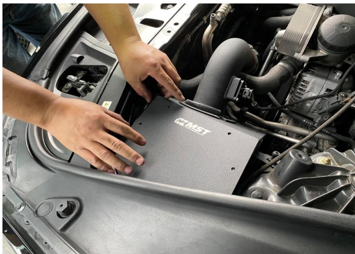
Figure 15: Install the heat shield cover.
