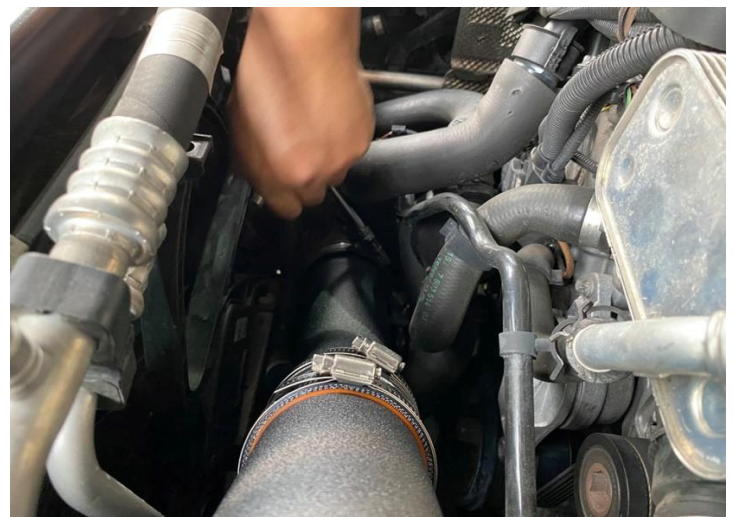
Figure 12: Tight the clamp.
