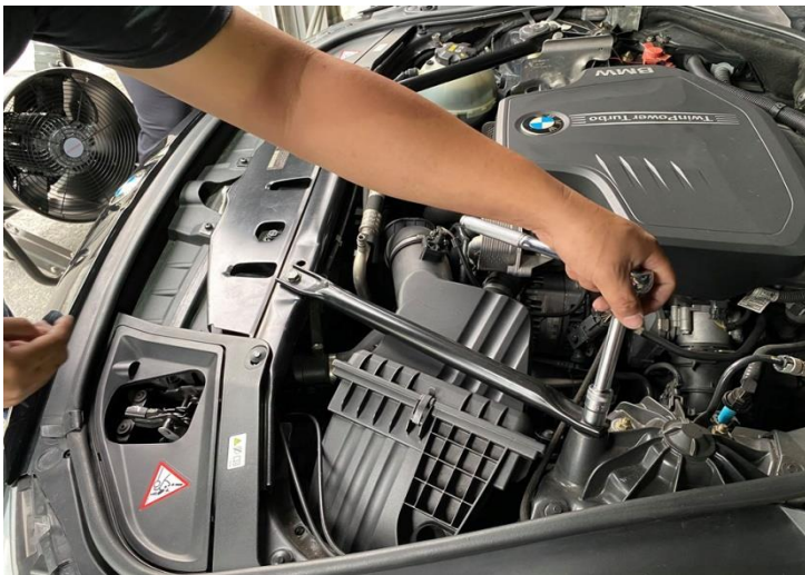
Figure 2: Remove the strut bar.
