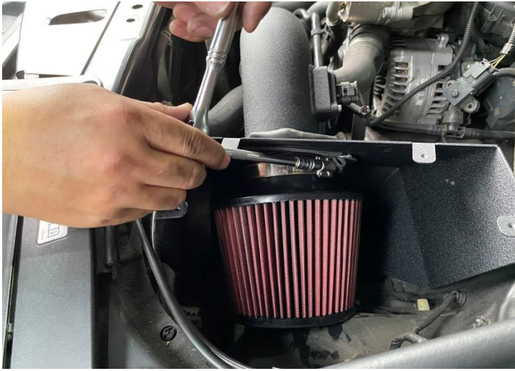
Figure 13: Install the air filter.
