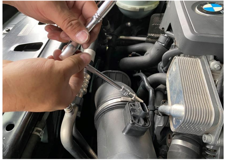
Figure 4: Loosen the stock tube clamp.
