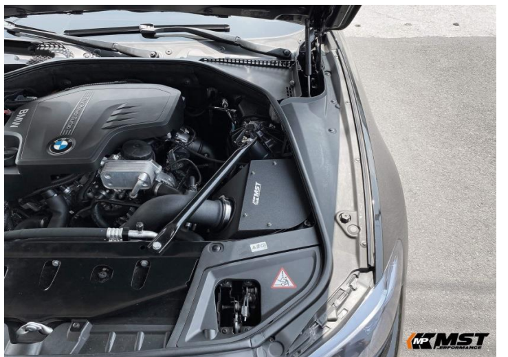
Figure 16: Install the strut bar.
