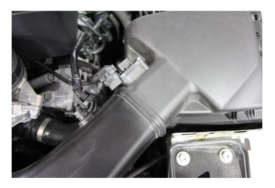
Step 2: Remove the factory air filter and bottom portion of the airbox. Pull straight up, it is held in by rubber grommets.
