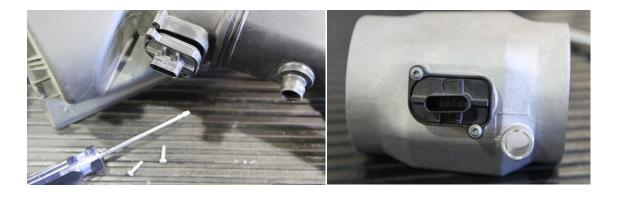
Step 8: Install the silicon coupler, MAF housing and the MAF support bracket (CTS-HS-800-3). Connect breather line, if equipped, otherwise leave the black cap cover on. Do not tighten clamps yet, adjust MAF housing until everything lines up perfectly. Take your time, this is a crucial step.
