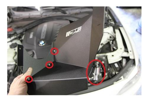
Step 5: locate and remove 8mm screw next to the strut tower. Install heatshield using the small screw you just removed and make sure mounting stud is installed in the factory grommet indicated by arrow.
