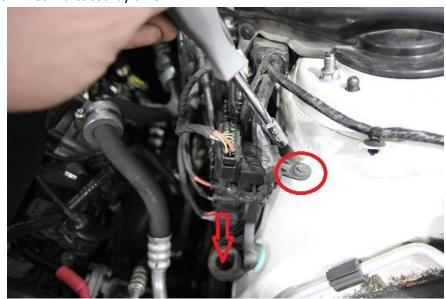
Step 6: Attach the front of heatshield using 10mm bolt and nut. There is a hole on the front where the heatshield will line up. Reach into the opening to secure the nut. Note: lower factory airduct will remain installed on the vehicle.
