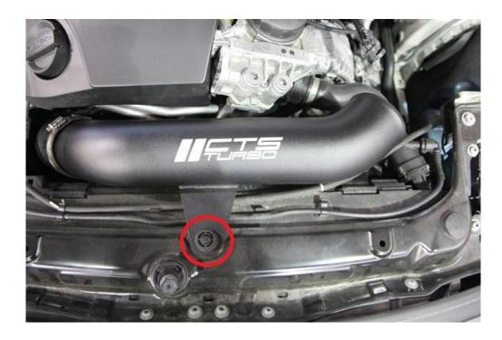
Step 4: Assemble the heatshield, CTS-HS-800-1 + CTS-HS-800-2 using supplied screws. Extra screws are included just in case. Note that smaller heatshield goes UNDER the larger one. Attach mounting stud with supplied 10mm bolt.
