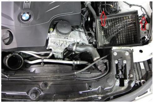
Step 3: Transfer the rubber grommet from the front of car onto the CTS intake tube. Install the intake tube CTS-IT-880 on the vehicle. Do not tighten clamp yet.
