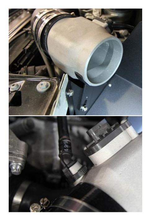
Step 9: Install the air filter – filter will rest on the support bracket and clamp will go around the support and filter securing both. Tighten all clamps (8 and 7mm) starting on filter side, work your way over to factory clamp, make sure you line up all the components as shown. Reconnect MAF harness. Start the car and let idle for 5-6 minutes. Test drive and you're done!
