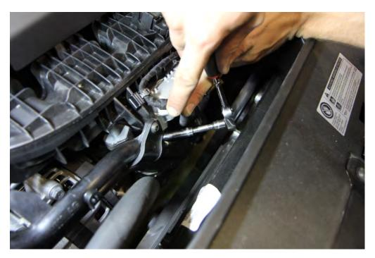
**Step 4:** Raise the car on jackstands or hoist. Use the T25 torx to remove the 8 screws holding the belly pan to the subframe.
