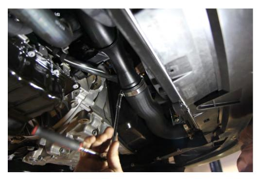
**Step 6:** Using the T30 Torx, undo the bottom bracket bolt holding the throttle pipe to the engine.
