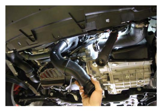
**Step 9:** Use the T20 Torx to remove the MAP sensor from the OEM pipe and use the supplied M6 allen bolts to reinstall in the supplied high flow pipe. Take note of the plug direction on the pipe. Utilize lubricant while reinstalling the MAP sensor into the new pipe to avoid tearing the o-ring. Use the 3/16 allen to install the supplied meth bung plug into the pipe.
