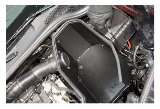
Step 10: Reinstall the pipe clamp on the intake pipe and plug in MAF sensor cable.
