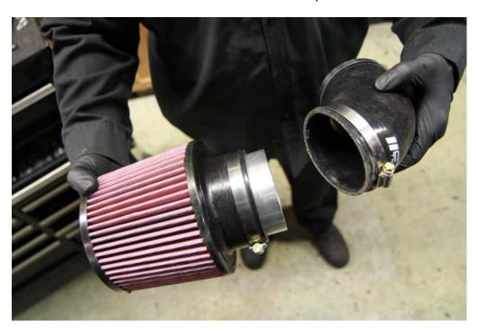
Step 12: Install the airfilter unit into the airbox. Reinstall front air ducting, tighten down the hose clamps. You are done!
