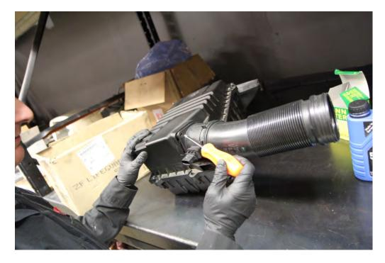
Step 6: Pull the 2 rubber grommets from the bottom of the airbox and reinstall on the new intake box. (if you have not yet assembled the airbox, do so now.)
