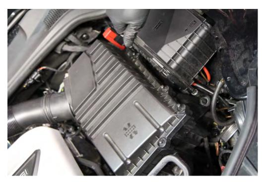
Step 5: Using a Philips screwdriver, undo the 2 screws holding the MAF housing to the airbox.
