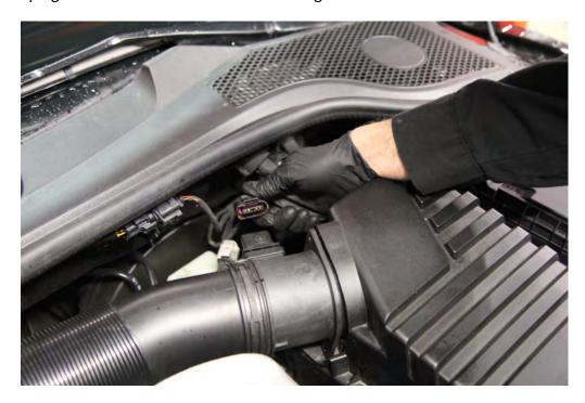
Step 2: Undo pipe clamp with the removal tool and slide towards passenger side.
