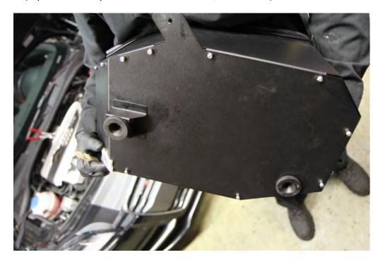
Step 7: Use the 10mm socket, install the OEM MAF housing to the intake box using the supplied 6mm bolts and nuts.
