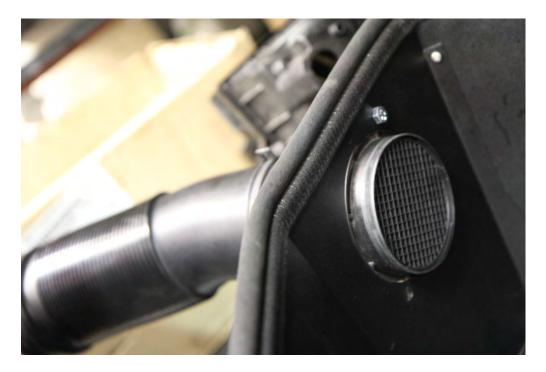
Step 8: Lubricate the rubber mounting points on the bottom of the airbox and press into the mounting points in the car. Note: hold mounting point under the airbox as shown to prevent flex.
