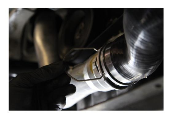
**Step 3**: Use the T30 Torx bit to remove the 2 bolts holding the outlet pipe to the engine.
