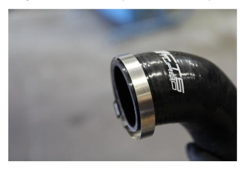
**Step 7**: Manouver the new pipe into place slipping the silicon over the new billet turbo hose adaptor. Reinstall the 2 T30 torx bolts and tighten the clamps over the silicon.
