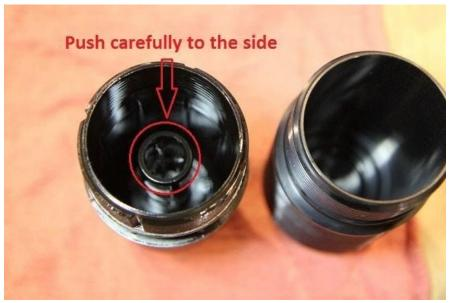
Carefully remove the filter cage by pushing it to the side of housing.
