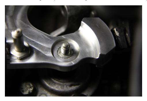
**Step 9**: Tighten the 13mm nut and confirm everything is connected. Inside the car, check the short shifter by shifting through ALL the gears. Make sure you are happy with the reduction in throw, change the pin position and test again.
