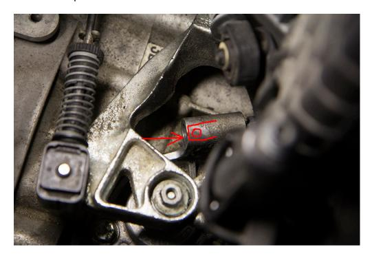
**Step 7**: Lift the cable end off its pivot pin. Take your 13mm ratchet and loosen the nut holding the shifter weight to the transmission.
