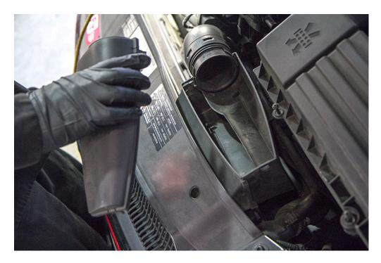
**Step 2**: Remove the MAF sensor cable by carefully undoing the clip. Using a pair of pliers, undo the spring clamp holding the MAF housing to the intake hose.
