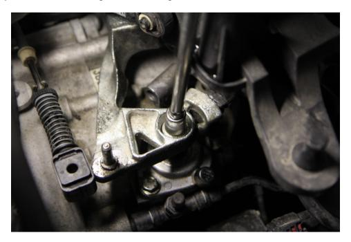
**Step 8**: Install the cable pin in the desired position. Outside bolt hole is 20% reduction. Inner bolt hole is 35% reduction. Align the splines of the weight with the transmission shaft spline.
