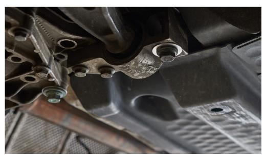
Control Arm Bracket Bolts M12 x 90 ---- 70 Nm (51 Ft-lbs) + 90 degrees Steering Rack Bolts M10 x 76 ---- 50 Nm (36 Ft-lbs) + 90 degrees Subframe Bolts - Lower M12 x 110 ---- 70 Nm (51 Ft-lbs) + 90 degrees Subframe Bolts - Upper M12 x 90 ---- 70 Nm (51 Ft-lbs) + 90 degrees
