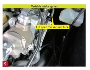
Secure the solenoid to any area in the engine bay, take note that the length of pipe B to the variable filter should not exceed 30cm
