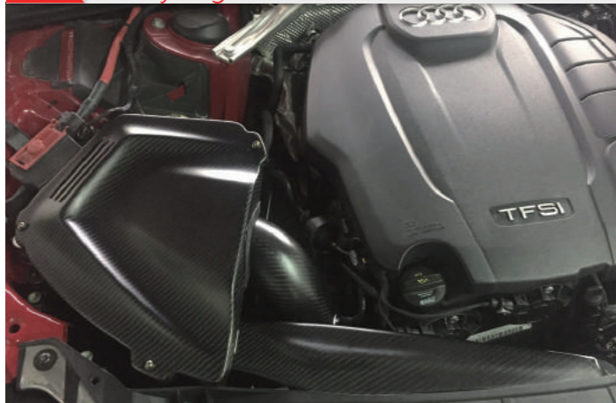
5 install the air box cover then re install the factory engine lid
